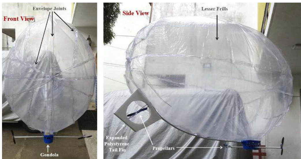
Figure 1: Front view (left image) and Side view (right image) of the implemented Blimp Robot
