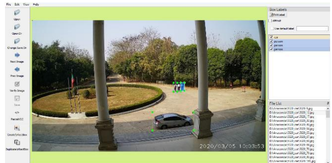
Fig. 3. Labeling images by using LabelImg tool
